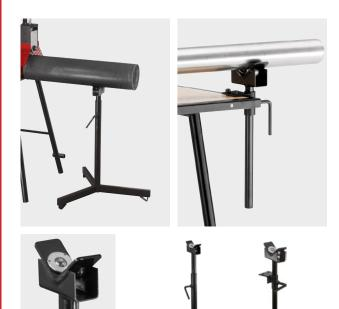
Robust, continuously height adjustable material rest with ball guide for pipes Ø ( $\frac{1}{2}$ )  $\frac{3}{4}$ –6", Ø (6) 26–115 mm, solid material Ø (6) 26–150 mm, load capacity up to 150 kg.
