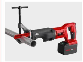
Powerful, robust, compact hybrid pipe saw for cordless and mains operation. Ideal for steel pipes and other pipes as well as for many materials, e.g. wood, wood with nails, pallets, metal, also stainless steel, cast iron, breeze blocks, plaster boards etc. Li-lon 22 V Technology! Li-lon 21.6 V, 9.0 Ah battery for approx. 80 1" steel pipe cuts with guide holder per battery charge\*.
