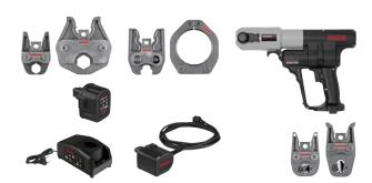
Robust, compact hybrid radial press 32 kN for cordless and mains operation, with automatic return (forced return). For radial press joints Ø 10–108 (110) mm, Ø ½–4". Li-lon 14.4 V, 5.0 Ah battery for approx. 450 pressings per battery charge\*.
