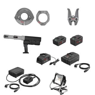
Powerful, universal, robust hybrid radial press XL 45 kN for cordless and mains operation with automatic circuit control. Antivibration system. For radial press joints XL Ø 64–108 mm, Ø 2½–4". Li-lon 22 V Technology! Li-lon 21.6 V, 5.0 Ah battery for approx. 150 pressings per battery charge\*.
