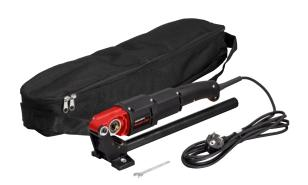
Handy, ultra light, robust electric pipe cutter for pipes of the pressfitting systems of stainless steel, C-steel Ø 12–28 mm, copper Ø 10–35 mm, composite tubes Ø 10–40 mm
