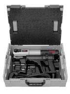
Robust, compact electric radial press 32 kN with automatic return (forced return). For radial press joints Ø 10–108 (110) mm, Ø 3/4–4"
