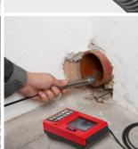
Very compact, lightweight, electronic camera inspection system for brilliant pictures and videos of pipes and drains Ø 40 – 150 mm, chimneys and other hollow cavities. Cordless and mains operation. With electronic metering. For documentation of pictures and videos on SD card.
