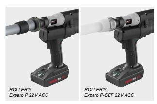
Ultra-handy, ultra-light, robust 20 kN hybrid pipe expander for cordless and mains operation, with automatic return (ACC). For expanding pipes/rings. Optionally with Cu, P or P-CEF expander. Li-lon 22 V Technology! Li-lon 21.6 V, 2.5 Ah battery for approx. 600 expansions per battery charge\*.
