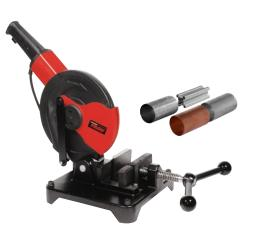
Powerful, compact. robust pipe circular saw especially for stainless steel pipes, carbon steel pipes and copper pipes of the pressfitting systems,  $\leq \emptyset$  76 mm. Also for cutting thin-walled profiles for before-wall installation.
