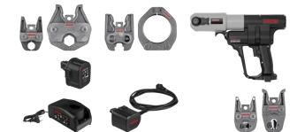
Robust, compact hybrid radial press 32 kN for cordless and mains operation, with automatic return (forced return). For radial press joints Ø 10–108 (110) mm, Ø  $\frac{1}{4}$ –4". Li-lon 14.4 V, 5.0 Ah battery for approx. 450 pressings per battery charge\*.
