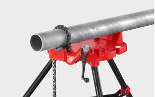
Robust pipe processing station with integrated chain pipe vice on collapsible tripod stand. For clamping pipes, solid material Ø  $\frac{1}{6}$  - 6", 10 – 165 mm. Load capacity up to 450 kg.
