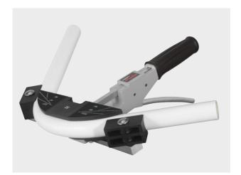
Practical, ultra handy, ultra light compact one-handed pipe bender for soft copper pipes Ø 10–22 mm, Ø %–%", s  $\le$  1.0 mm, soft jacketed copper pipes Ø 10–18 mm, Ø %–%", s  $\le$  1.0 mm, soft coated carbon steel pipes of the press fitting systems Ø 12–18 mm, s  $\le$  1.2 mm, soft precision steel pipes Ø 10–18 mm, s  $\le$  1.0 mm. Multi-layer composite pipes Ø 14–32 mm. (s = wall thickness)
