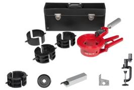
Robust pipe cutting and pipe chamfering device made of metal for right-angled, flat cutting and chamfering (15°) of plastic tubes of ABS, PB, PE, PE-HD, PE-X, PVC, PVDF, Ø 40–110 mm.
