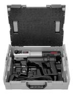
Robust, compact electric radial press 32 kN with automatic return (forced return). For radial press joints Ø 10–108 (110) mm,  $\emptyset$   $^{3}$ –4"
