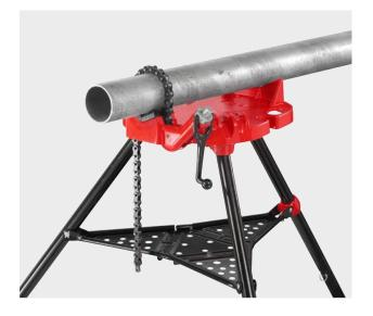
Robust pipe processing station with integrated chain pipe vice on collapsible tripod stand. For clamping pipes, solid material Ø  $\frac{1}{6}$ -6", 10–165 mm. Load capacity up to 450 kg.
