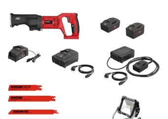
Powerful, robust, compact hybrid universal reciprocating saw for cordless and mains operation. For sawing numerous materials such as wood, wood with nails, pallets, metal, also stainless steel, cast iron, breeze blocks, plaster boards, pumice stone, clinker and brick. Ideal for sawing steel pipes and sections. Li-lon 22 V Technology! Li-lon 21.6 V, 5.0 Ah battery for approx. 75 1" steel pipe cuts per battery charge\*.
