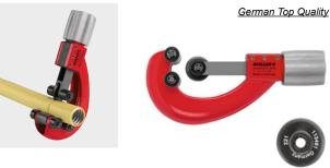
Compact, robust, quality pipe cutter with needle-bearing-mounted cutting wheel and counterpressure rollers, especially for corrugated metal hoses (corrugated pipes) made of stainless steel, also jacketed, DN 10–32 (40), Ø ¾–1½" (2").
