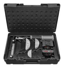
Compact, robust, oil-hydraulic hybrid pipe bender for cordless and mains operation. For soft copper pipes Ø 10-22 mm, Ø %-76",  $s \le 1.0$  mm, soft coated copper pipes Ø 10-18 mm, Ø %-56",  $s \le 1.0$  mm, pipes of the pressfitting systems made from stainless, nickel steel Ø 15-22 mm,  $s \le 1.2$  mm, made from soft carbon steel, coated Ø 12-18 mm,  $s \le 1.2$  mm, soft precision steel pipes Ø 10-18 mm,  $s \le 1.5$  mm. Multilayer composite pipes Ø 14-32 mm. (s = wall thickness)
