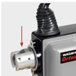
Clamping jaws outside the housing!
