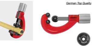
Compact, robust, quality pipe cutter with needle-bearing-mounted cutting wheel and counterpressure rollers, especially for corrugated metal hoses (corrugated pipes) made of stainless steel, also jacketed, DN 10-32 (40), Ø %-1½" (2").
