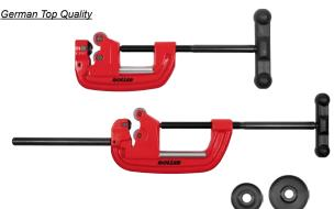
Robust, quality pipe cutter for steel pipes Ø  $\frac{1}{6}$ -4", Ø 10-115 mm, wall thickness s  $\leq$  12.5 mm.
