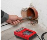
Very compact, lightweight, electronic camera inspection system for brilliant pictures and videos of pipes and drains Ø 40 - 150 mm, chimneys and other hollow cavities. Cordless and mains operation. With electronic metering. For documentation of pictures and videos on SD card.
