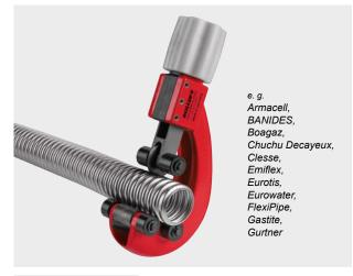
Compact, robust, quality pipe cutter with needle-bearingmounted cutting wheel and counterpressure rollers, especially for corrugated metal hoses (corrugated pipes) made of stainless steel, also jacketed, DN 10–32 (40), Ø  $\frac{3}{8}$ –1 $\frac{1}{2}$ " (2").
