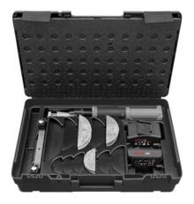
Compact, robust, oil-hydraulic hybrid pipe bender for cordless and mains operation. For soft copper pipes Ø 10–22 mm, Ø %–%", s ≤ 1.0 mm, soft coated copper pipes Ø 10-18 mm, Ø %-5/8'  $s \le 1.0$  mm, pipes of the pressfitting systems made from stainless, nickel steel Ø 15–22 mm, s ≤ 1.2 mm, made from soft carbon steel, coated Ø 12-18 mm, s ≤ 1.2 mm, soft precision steel pipes Ø 10−18 mm, s ≤ 1.5 mm. Multilayer composite pipes Ø 14-32 mm. (s = wall thickness)
