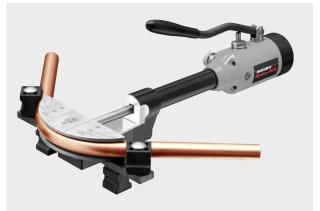
Effortless, oil-hydraulic manual pipe bender for soft copper pipes Ø 10-22 mm, Ø 36-76", s  $\leq 1.0$  mm, soft coated copper pipes Ø 10-18 mm, Ø 36-56", s  $\leq 1.0$  mm, pipes of the pressfitting systems made from stainless, nickel steel Ø 15-22 mm, s  $\leq 1.2$  mm, made from soft carbon steel, coated Ø 12-18 mm, s  $\leq 1.2$  mm, soft precision steel pipes Ø 10-18 mm, s  $\leq 1.5$  mm. Multilayer composite pipes Ø 14-32 mm. (s = wall thickness)
