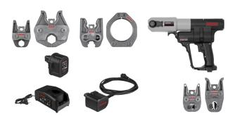
Robust, compact hybrid radial press 32 kN for cordless and mains operation, with automatic return (forced return). For radial press joints Ø 10–108 (110) mm, Ø  $\frac{1}{4}$ –4". Li-lon 14.4 V, 5.0 Ah battery for approx. 450 pressings per battery charge\*.
