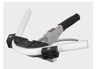
Practical, ultra handy, ultra light compact one-handed pipe bender for soft copper pipes Ø 10–22 mm, Ø  $\frac{3}{6}-\frac{7}{6}$ ", s  $\leq$  1.0 mm, soft jacketed copper pipes Ø 10–18 mm, Ø  $\frac{3}{6}-\frac{5}{6}$ ", s  $\leq$  1.0 mm, soft coated carbon steel pipes of the press fitting systems Ø 12–18 mm, s  $\leq$  1.2 mm, soft precision steel pipes Ø 10–18 mm, s  $\leq$  1.0 mm. Multi-layer composite pipes Ø 14–32 mm. (s = wall thickness)
