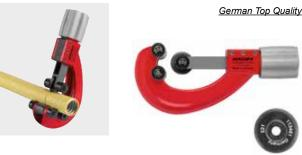
Compact, robust, quality pipe cutter with needle-bearing-mounted cutting wheel and counterpressure rollers, especially for corrugated metal hoses (corrugated pipes) made of stainless steel, also jacketed, DN 10-32 (40),  $\emptyset$   $\frac{3}{2}$ -1½" (2").
