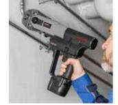
Robust, compact hybrid radial press 32 kN for cordless and mains operation, with automatic return (forced return). For radial press joints Ø 10–108 (110) mm, Ø ¼–4". Li-Ion 14.4 V, 5.0 Ah battery for approx. 450 pressings per battery charge\*.
